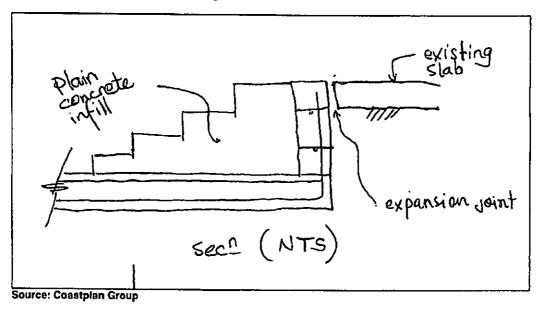
It should be noted that the waterproof membrane will need to extend under the proposed step structure and link to the membrane under the existing slab where the stairs join the existing.
