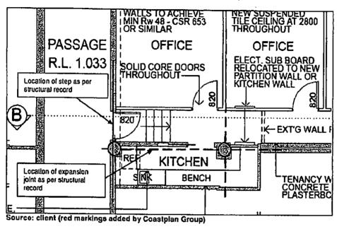
Based on the structural record the existing floor slab is considered an infill slab between the columns. The following sketch shows the extent of the section of the slab to be removed.
